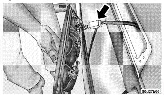
3. Turn desired bulb socket 1/4 turn and remove socket and bulb from housing.
